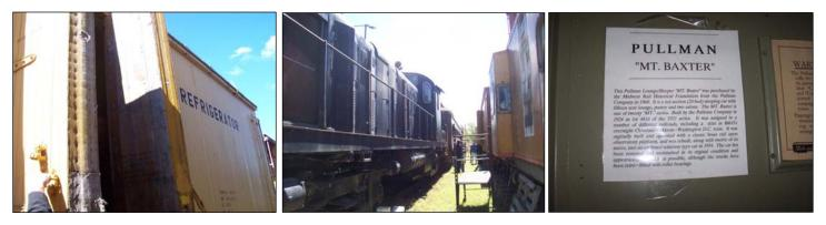
that I can remember seeing how thick the doors and car walls were. This car would have the ends filled with ice and compartmentalized with fans to distribute the cool air to keep the produce fresh. The fans ran from generators on the trucks of the car. The railroad would put these trains on the green light and even the passenger trains waited for the produce trains to come through as the railroad did not want to pay for the spoilage.
