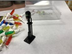
block signals that will accept the 2mm LEDs. The blue LEDs could be used to simulate welding and the yellow make pretty good freeway street lighting or interior building
