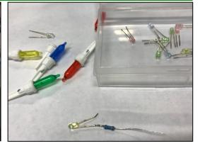
pull the colored cover off you'll find a 2mm LED having a slight tint indicating the color it will produce when lit. Using a 330 ohm 1/4 watt resistor in series it will operate from a 12 volt source.
