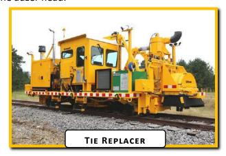
The Kershaw® Model 47-6 Tie Replacer can remove or insert wood or concrete ties up to 18 feet long. The puller/inserter head operates on a slewing ring to allow functionality and versatility from either side of the track, without turning the machine. Rail lifters grip and lift the rail for tie insertion or removal. The rail lift height is automatically controlled for
