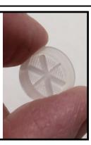
What I am left with is the larger tube and the small end cap. Both of these have tiny perforations on the ends. They also have ribs inside that sort of look like fan blades.
